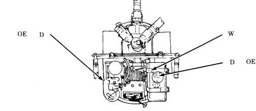
Crankcase Drain Plug (Drain and refill)
